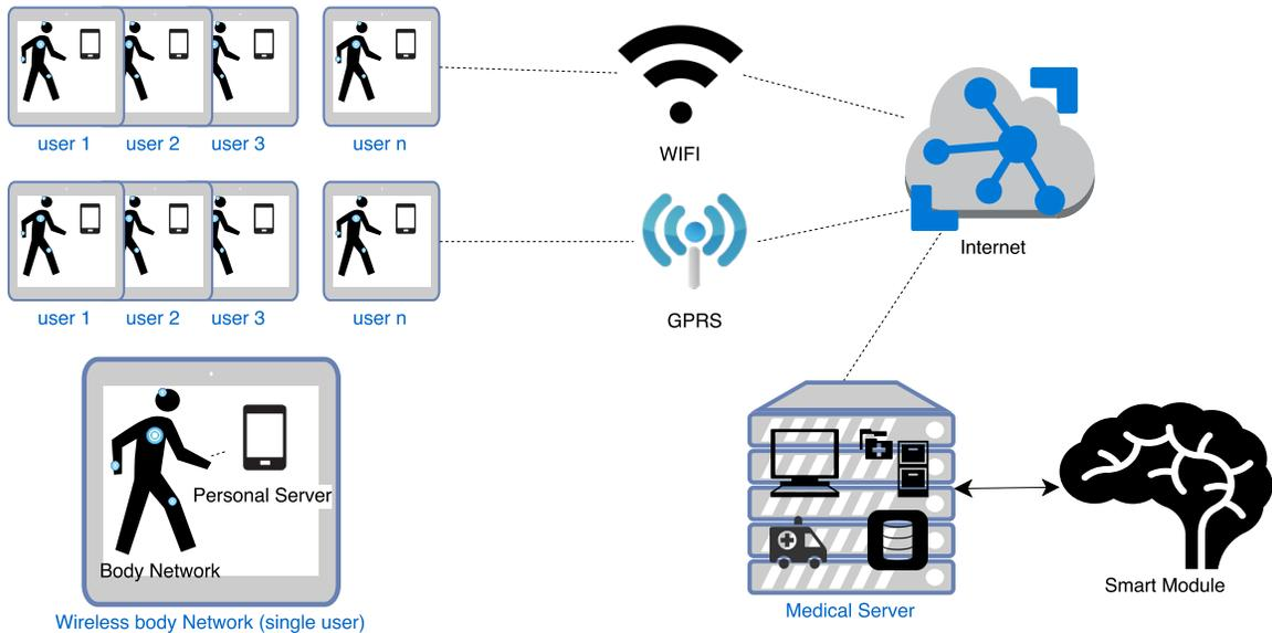
Fig. 2: Illustration of Continuous Monitoring Architecture with Proposed Smart Module
